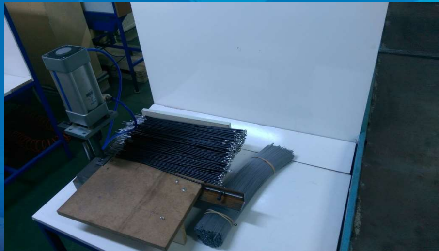
Terminal pressing on wire ropes
